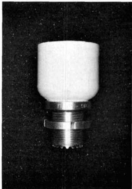
fig. 2. PVC pipe cap with the UG-266/U coax connector installed.
